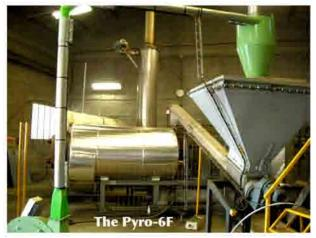
In 2002 Pro-Natura won the Altran Foundation's first prize for technological innovation with its pioneering pyrolysis unit, the Pyro-6F. That machine shows that it is possible to make a form of "green charcoal" from carefully selected and otherwise unused agricultural and/or forestry wastes in a highly ecological and efficient manner. Its cycle is:
